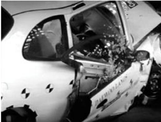
Offset crash test at 64km/h
